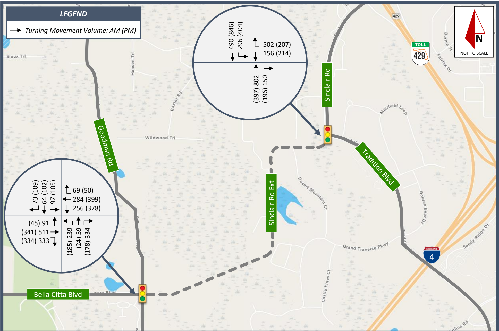
Exhibit 10: Horizon Year (2045) Intersection Turning Movement Volumes Sinclair Road Extension | Preliminary Traffic Evaluation
