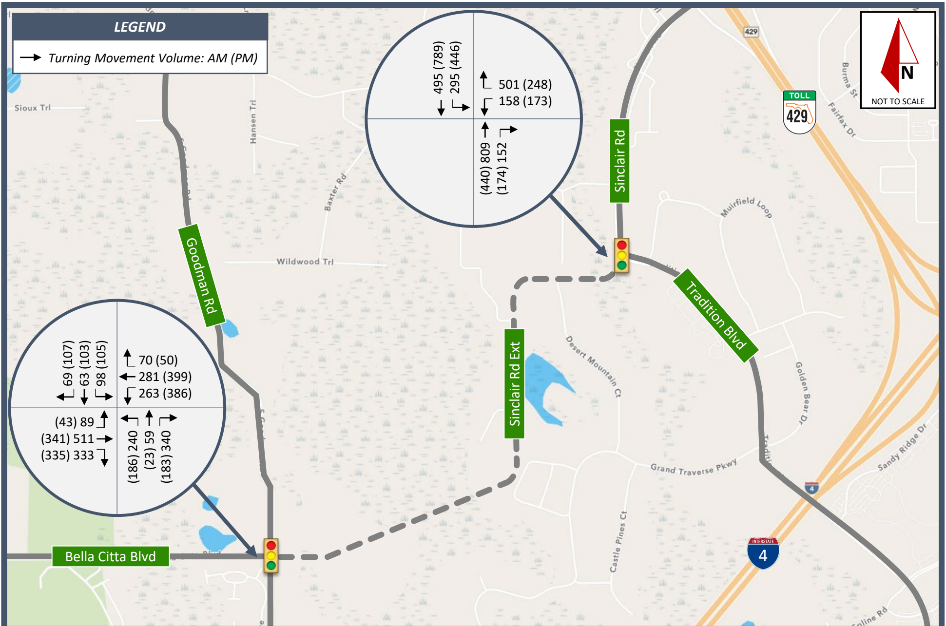
Exhibit 10: Design Year (2045) Build Intersection Turning Movement Volumes Sinclair Road Extension | Project Traffic Analysis Report (PTAR)
