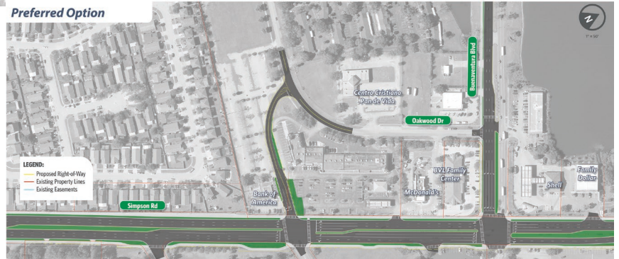
Phase 4: 125 ft of Right-of-Way with 4 Traffic Lanes and 2 Auxiliary Lanes
