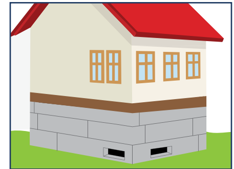
Finished foundation walls with flow-through openings. House is lowered down on to the new walls.
