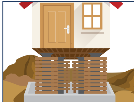
Home is slowly raised by hydraulic jacks and temporary cribbing installed underneath.
